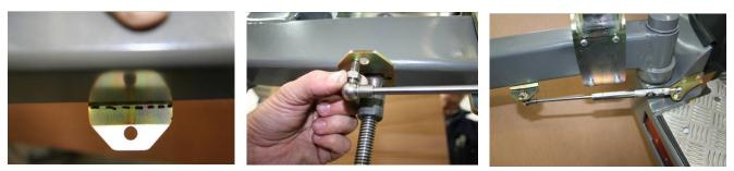
Note: With this bracket clamped into position, a measurement of 275mm should be achieved between the two hole centres of each bracket.
