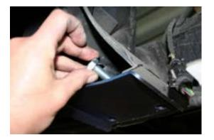
7. If the rear most hole in the chassis has a crush tube fit M12 x 110 x 1.75 bolt with flat washer through the bar and crush tube.
