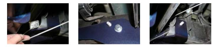
6. Fit M12 x 1.75 x 30 bolt through top of spring hanger, down through plate at end of pipe gusset. Secure using M12 flat, spring and nut. **TIGHTEN ALL BOLTS.**
