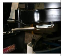
strut fits through from the underside of the tab on the carrier arm. Attach using M8 nyloc nut. Leave loose.
