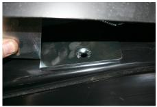
4. Fit the second bolt on wire through the same hole in the chassis up to the remaining hole in the bracket. Secure using M8 spring washer and M8 Nyloc nut.
