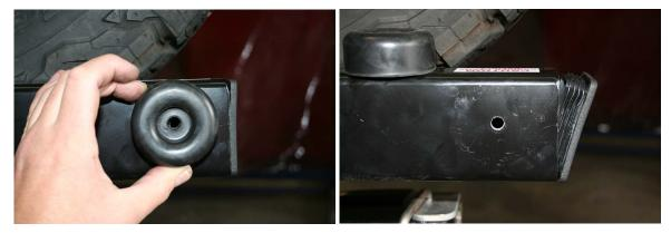
3. Remove the end cap and fit the bump stop using M10 x 1.5 x 30 bolt, spring and flat washers and wizz nut.
