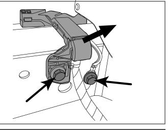
Release wiring loom from RH body bracket by un-clipping
