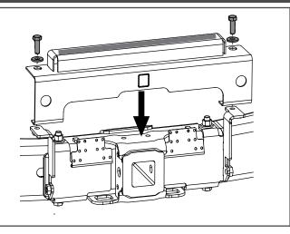
Loosely install LH swing arm assembly, ITEM 16, as shown using 3x M12 nuts & 3x M12 washers in upper positions and 2x M12x40 bolts & 2x M12 washers in lower positions, ITEMS 53, 56 & 50
