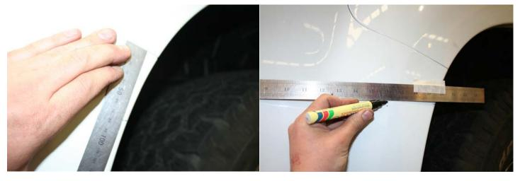
11. From the top of the bumper above the two sensor holes mark down 50mm, the mark should be about 3/4 of the way through the top of the sensor holes. Join the lines using a ruler
