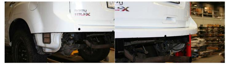
13. Fit pinchweld supplied to the bumper starting form the wheel arch around to the oppopsite side. The pinchweld should cover the two centre sensor holes (refer Fig 22)
