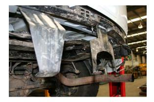
8. Refit bumper to the vehicle clipping in place and making sure it sits in its original position
