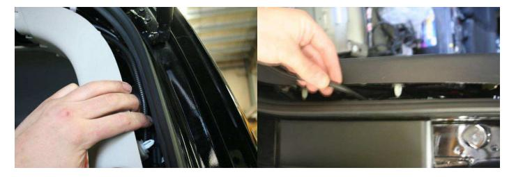
5. Remove small rubber grommet on outside of body. Feed wiring though hole until new grommet comes through and secure grommet in hole.
