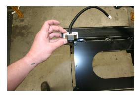
13. Plug in the patch harness under the vehicle. Then feed the wiring up to the carrier arm. Using cable tie mounts and cable ties run the harness along the bottom of the arm to the camera. Fit heat shrink and plug in the camera.
